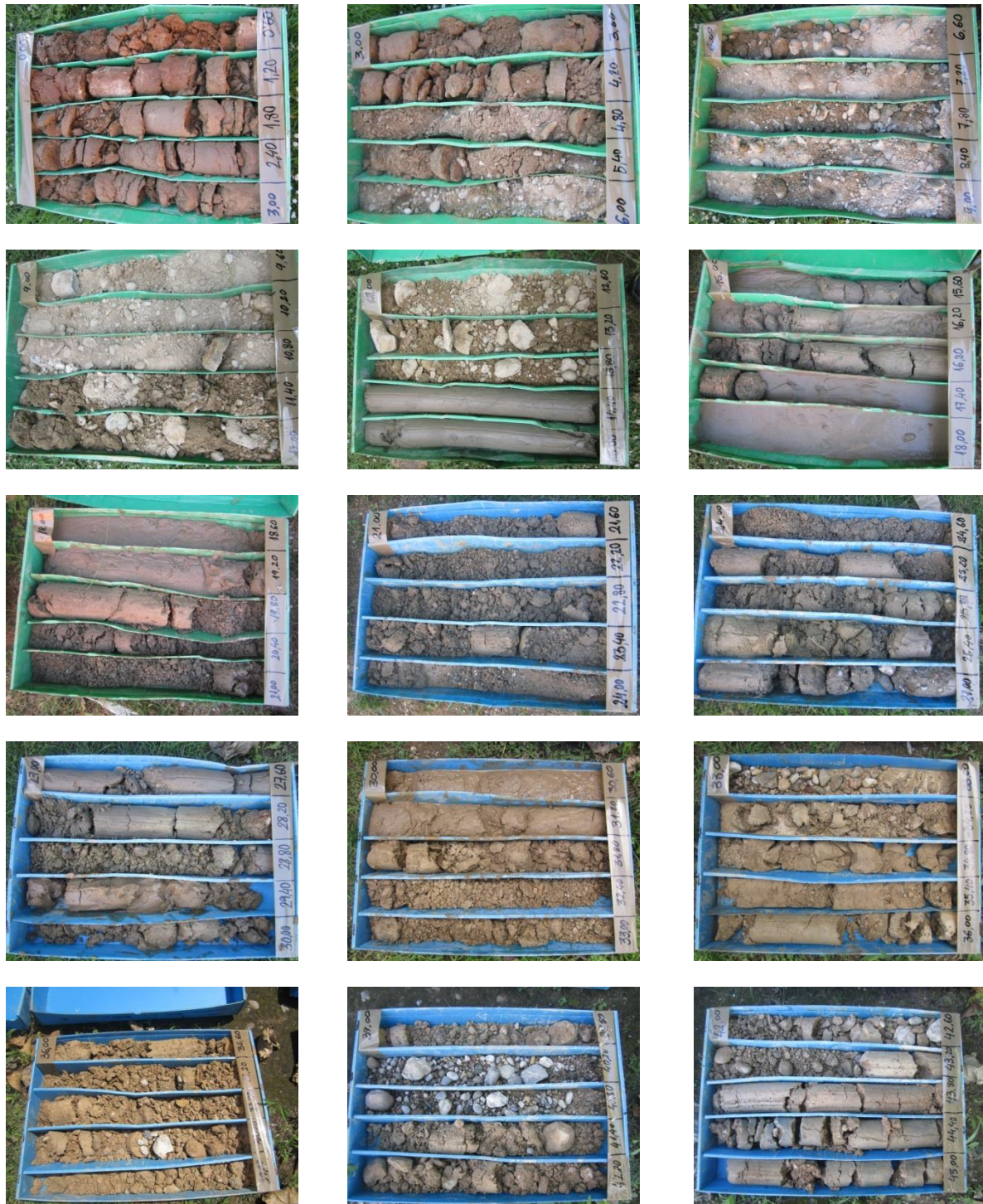
Figure 27: Total set of storage boxes Pz1 (continuous drilling) Note: each box has a total storage of 3 meters of sediments
