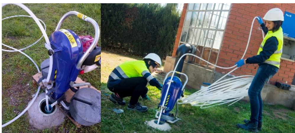
Figure 19: Water sampling procedure at SJD control piezometers
